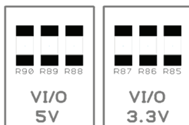
Figure 7-1 : PCI Signal Voltage Configuration Resistors (Bottom View)
